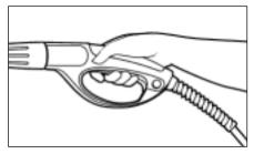
Step 3 Turn on the pressure washer. Pull trigger to operate unit: Liquid detergent is drawn into the unit and mixed with water. Apply detergent to work area. Do not allow detergent to dry on surface. For best results see Cleaning Tips on pages 8 & 9 for specific information on how to clean different surfaces.
